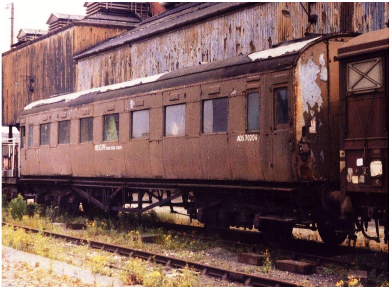
S 1319 S, similar to, and from the same batch as 1323 and 1346; in departmental condition as ADS 70206 at South Lambeth Goods Depot, note the 2 louvre vents over the toilet window, 30/5/80
