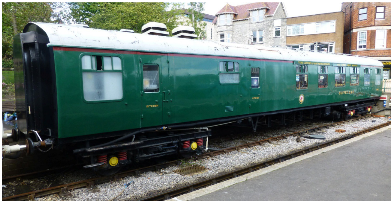
S 1947 in service at Swanage in its new position in the 'Squint' on 23 rd May 2014. This shows the kitchen side and the B4 bogies.
