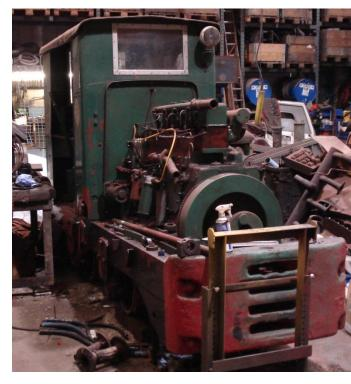
The engine, gearbox and fuel system have had a thorough overhaul with new cylinder liners and pistons fitted. The loco will require further work to the bodywork and new horn and lights to be fitted, but at present it is in running order. It is the same model of locomotive as once could be seen crossing the A351 and Skew Bridge in the 1950's and 60's
