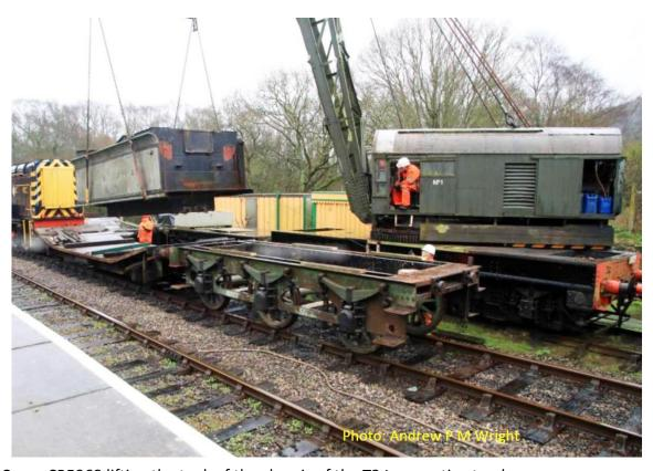
Crane CB5968 lifting the tank of the chassis of the T3 Locomotive tender
