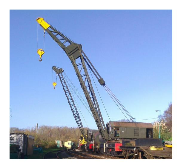
The two cranes which are often seen in the siding opposite the platform at Norden Station were built in the late 1940s and early 1950s by Stothert and Pitt of Bath for use at the Southampton Docks. These cranes are known on the Swanage Railway as FBC1 and FBC2 but officially the makers numbers are CB5968 No1, 15 ton; and CC1011 No1 10 ton, respectively.
